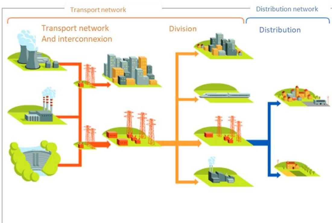
**Figure 1:** Transmission (high voltage) and distribution (medium voltage) and dispensing (low voltage) network of the power grid.
